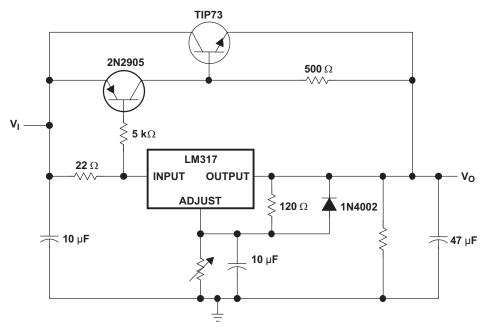
Figure 23. High-Current Adjustable Regulator Circuit
