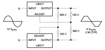
Figure 20. AC Voltage-Regulator Circuit
