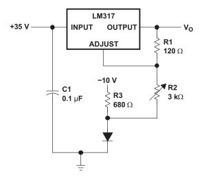
Figure 12. 0-V to 30-V Regulator Circuit
