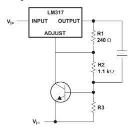
Figure 21. Current-Limited 6-V Charger Circuit
