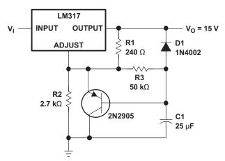
Figure 19. Slow Turn-On 15-V Regulator Circuit
