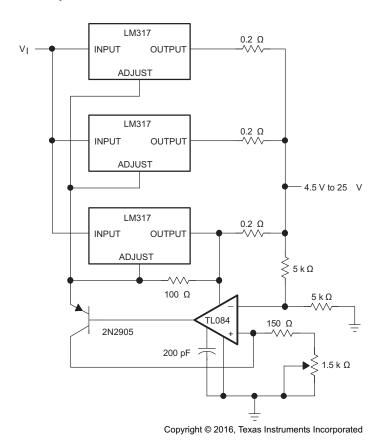
Figure 22. Adjustable 4-A Regulator Circuit
