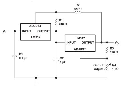
Figure 15. Tracking Preregulator Circuit
