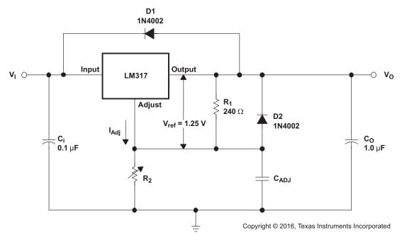
Figure 9. Adjustable Voltage Regulator
